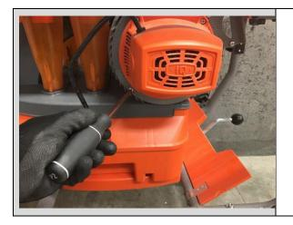
4. Unscrew vacuum screws and remove vacuum
