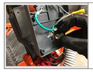
10. Route the wires through the opening at the bottom of the base of the control module
