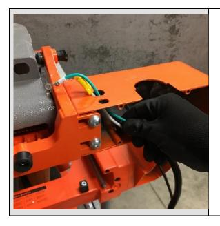
16. Route the saw motor power cable through the opening.
