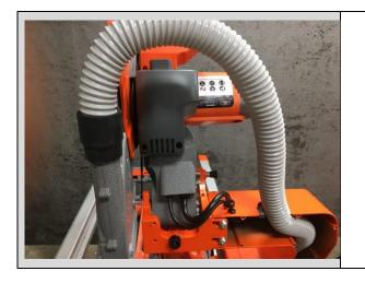
1. Connect the vacuum hose on to the inner dust guard
